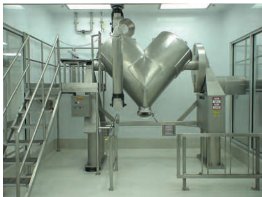
FIGURE 6.2 Industrial-size solid-state processor or twin shell blender used to mix solid particles. (Courtesy of Abbott Laboratories.)
