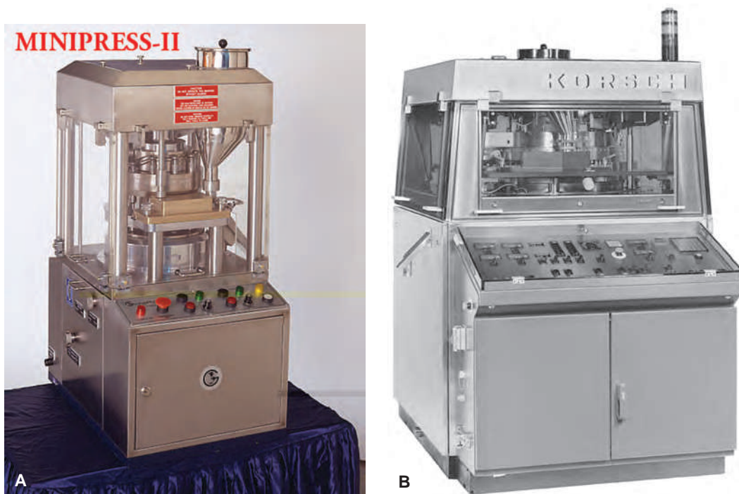
FIGURE 8.1 A: MiniTablet Press for development and small-scale production. (Courtesy of GlobePharma.) B: High-performance double rotary tablet press. The Korsch PharmapressR has a maximum output of 1 million tablets per hour, but for continuous operation, it is generally run to produce 600,000 to 800,000 tablets per hour. (Courtesy of Korsch Tableting.)
