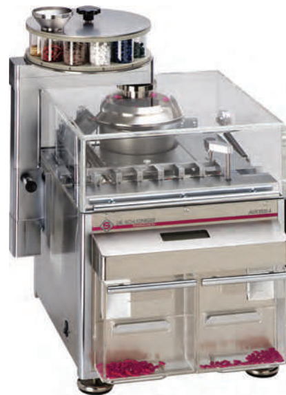
FIGURE 8.12 Automatic weight, hardness, thickness, and tablet diameter test instrument for quality control. Using a microprocessor and monitor for visualization, the instrument can test up to 20 samples at a time. (Courtesy of JB Pharmatron.)
