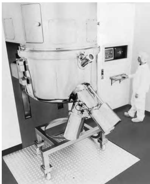
FIGURE 8.22 Microwave vacuum processing in which tablet ingredients are dry mixed, wetted with a binding liquid, and dried by vacuum and microwave in a single piece of equipment. (Courtesy of GEI Processing.)
