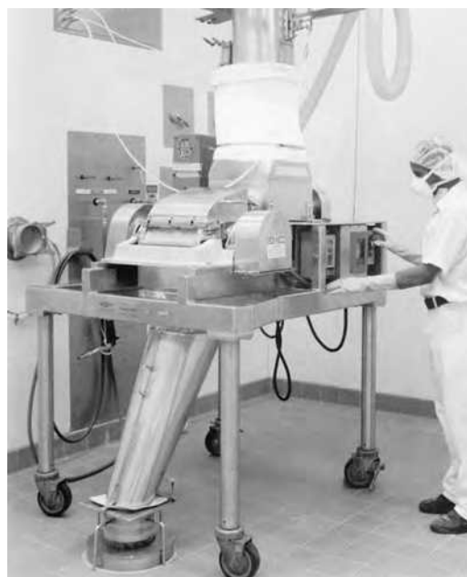
FIGURE 8.23 Frewitt Oscillator or Fitz Mill used to pulverize or granulate. (Courtesy of Eli Lilly and Company.)
