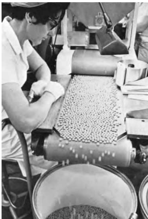
FIGURE 8.37 Checking for physical imperfections in coated tablets. (Courtesy of Smith, Kline & French.)
