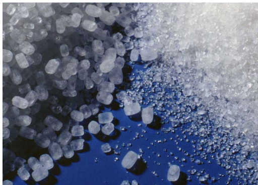
Figure 6.1 Different samples of bulk (\text{NH}_4)_2\text{SO}_4 -crystals from continuous crystallization with fines dissolution (left) and without fines dissolution (right).
