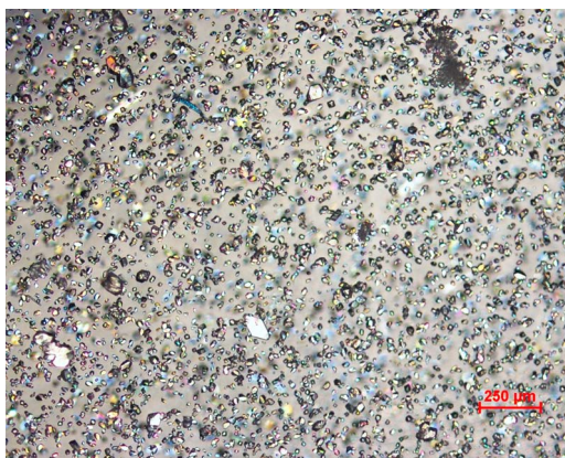
Figure 1.9 Deposited crystals on the surface of the polymeric excipient film from a continuous process.
