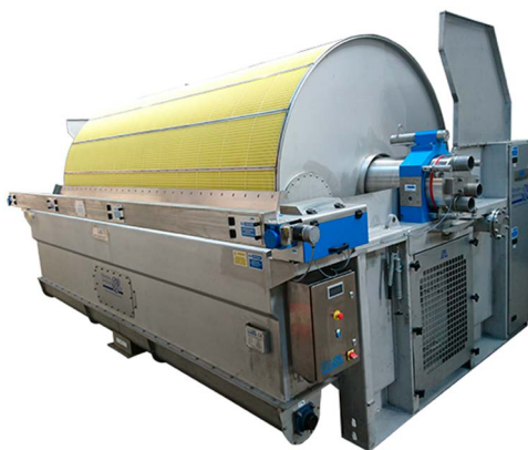
Figure 13.12 Rotary drum vacuum filter (RDVF). Image courtesy of Filtration Services Ltd.
