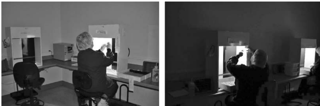
Figure 22-2 Manual visual inspections. Source: Courtesy of Baxter Healthcare Corporation.
