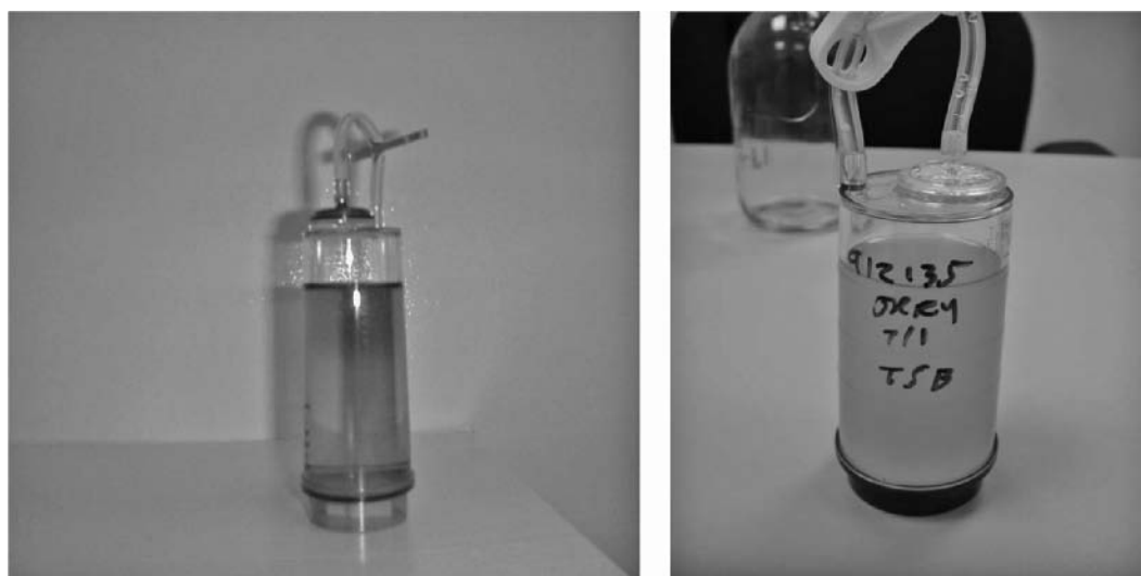
Figure 27-1 (Left) Sterile fluid thioglycollate medium (Right) non-sterile trypticase soy broth. Source: Courtesy of Ryan Cool, Baxter BioPharma Solutions.
