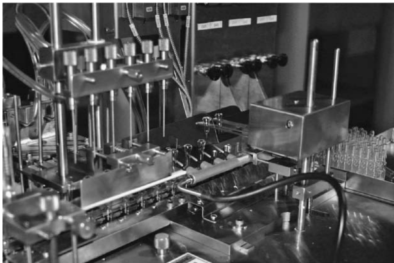
Figure 19-10 FPS1 automatic monoblock ampoule filling and sealing machine. Source: Courtesy of Cozzoli Machine Company.
