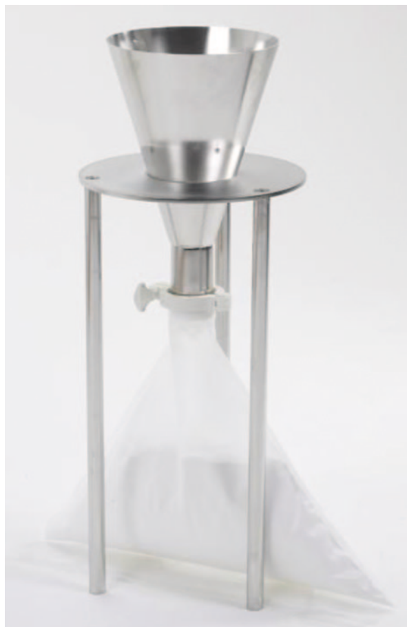
Fig. 7 Contained transfer of freeze-dried powder product to the LDPE bag by means of a hopper. LDPE low-density polyethylene (Image courtesy: ATMI Life Sciences)
