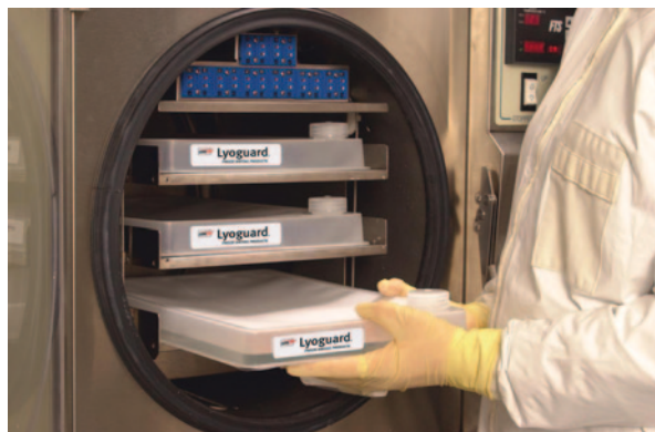
Fig. 10 GORE® LYOGUARD® trays as loaded for a freeze-drying cycle. (Courtesy W. L. Gore & Associates, Inc., Elkton, MD, USA; GORE, LYOGUARD and designs are trademarks of W.L. Gore & Associates)
