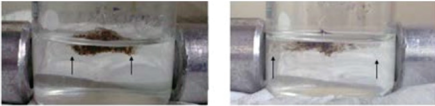
Fig. 21. CMC-NP hydrogel between two opposing permanent magnets at the beginning of the test (to the left) and after some hours (to the right).
