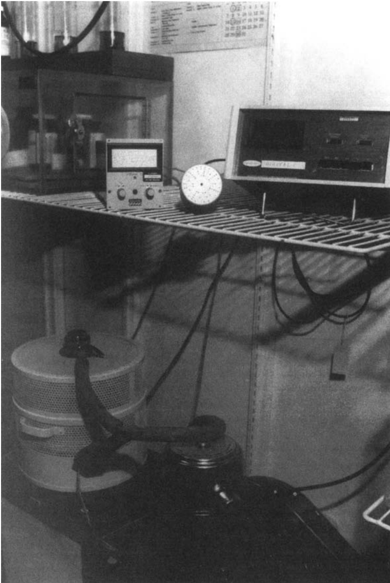
FIGURE 2 Vacuum pump, Pirani vacuum gauge, and hygrometer in low-humidity room for gravimetric moisture test.
