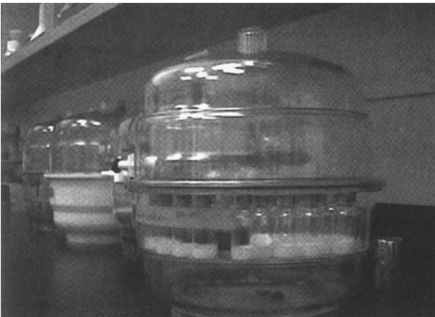
FIGURE 8 A demonstration of conducting a moisture sorption study with desiccators.
