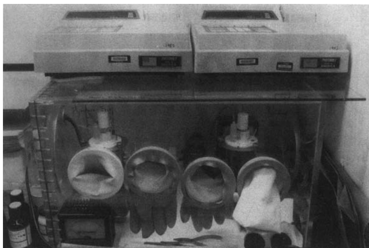
FIGURE 5 Karl Fischer dry box configuration with coulometric processing unit outside and titration vessels inside the dry box. Elongated wires connect the instrument to electrodes in the titration vessel in the dry box. Unit on the right uses pyridine solvent; unit on the left uses pyridine-free solvent.
