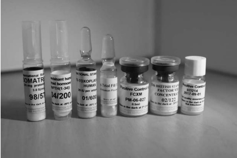
FIGURE 1 Lyophilized biological reference materials produced at NIBSC, showing 5-mL and 3-mL ampoules, crimp topped, and screw-capped vials.
